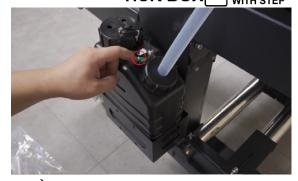
Put the waste ink tubes(the small one) into the waste ink hose
