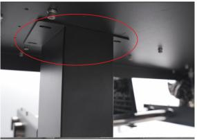
Tighten the fixing screws on both sides
