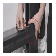
Turn around and install the second bar. Make sure to align with the holes in red circle
