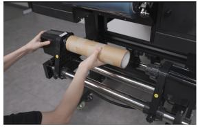
**Install the A film**Install the A film, tighten the knobs when center the A film with B film.
