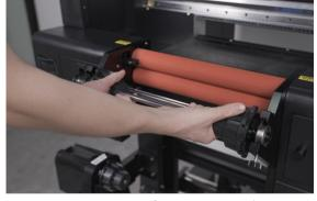
Take out the bracket of B film, Remove the holder from one side,
