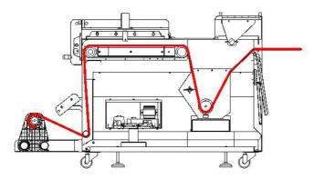
Lead the material to be solidified to the bottom of the powder box into the shaking powder bar above and between the platform for solid color, and finally roll the solid color material into the receptacle barrel or through the guide belt and the guide belt suction will bring out the print screen for printing while planting cut.
