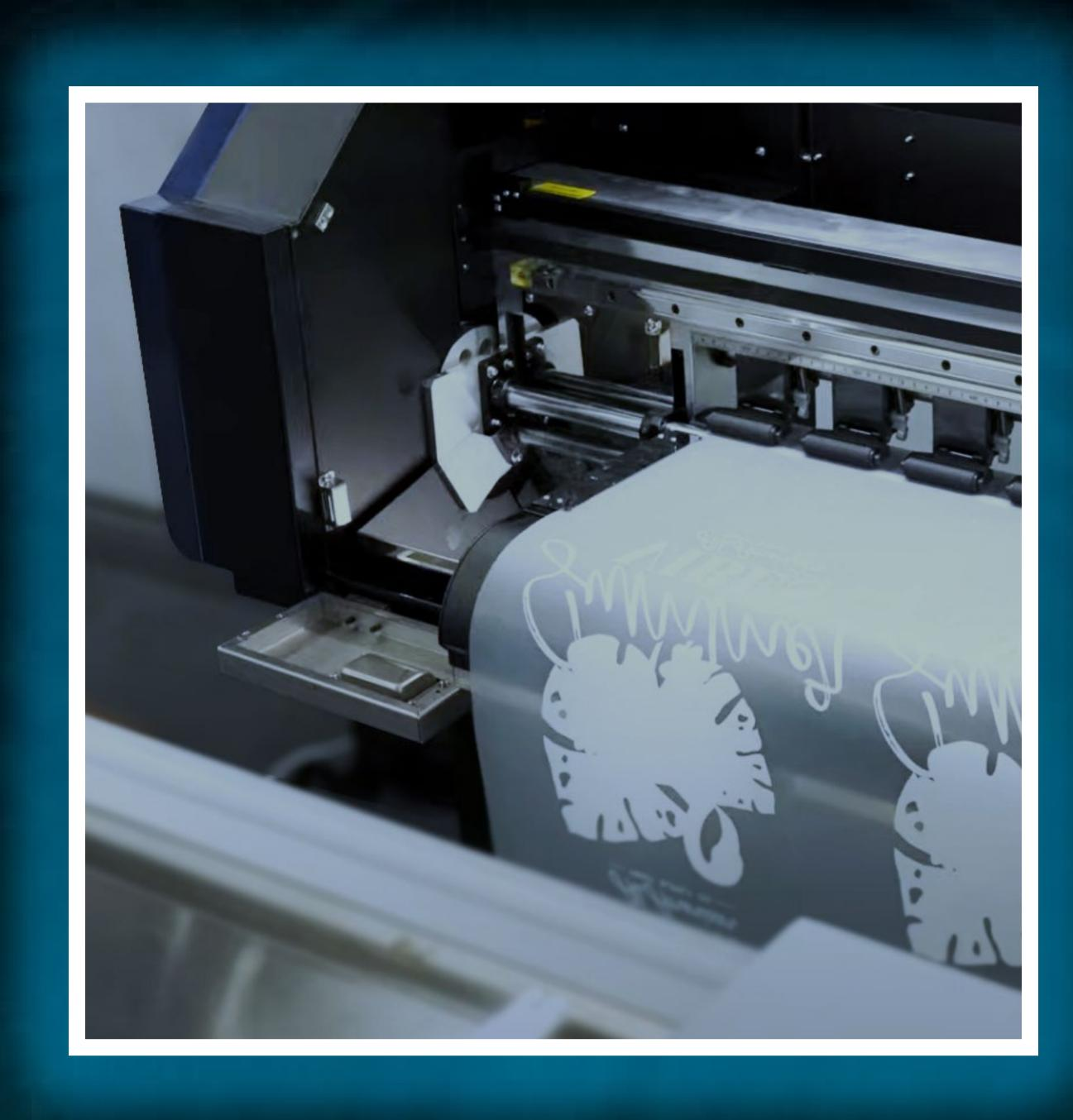
Smart Feed Reel, Sensor to Drive substrate to the printer without slipping
