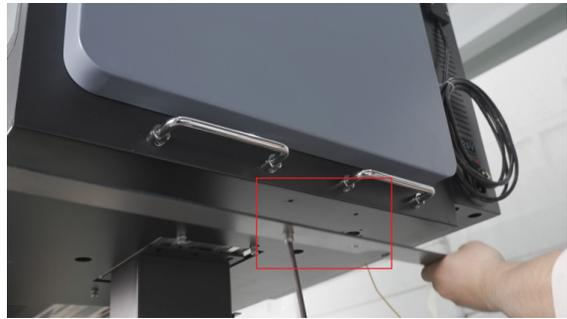
Tighten the screws underneath the printer body with the stand.
