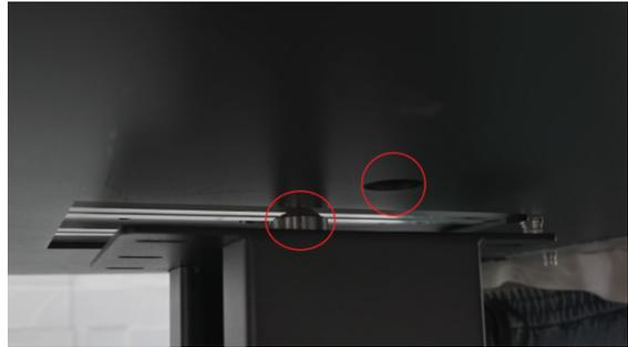
Remove the metal piece at the bottom of the printer body.
