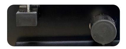
6. The last step is to add the empty roll to the holder and adjust it so that the film from the printer is straight and well aligned when it is attached to the empty roll it comes time to print. You want to be sure that the film does not sag on either side when it is connected to the end roll. Once you are happy with the alignment, tightening the knobs on the front of the roll holders to keep them secured in place.
