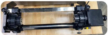
5. At this point, the tube end caps can be attached and the motor can be plugged into the port located on the right-hand side of the shaker unit.
