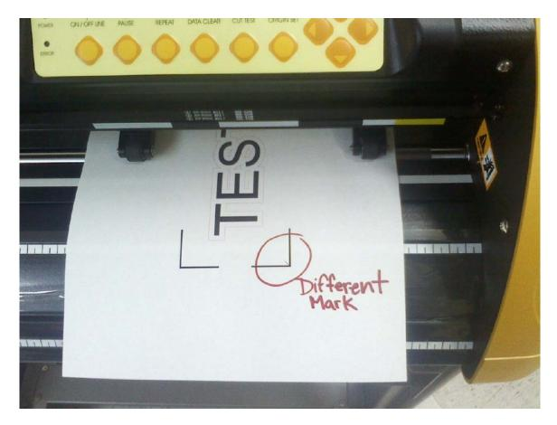
Load print out into machine, size up material, take machine offline and move cutting head directly over the first mark corner, push origin set, and back online.
